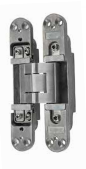
Shown Less Cover Plates less than 80KG with 3 hinges per door up to 1000mm wide door
